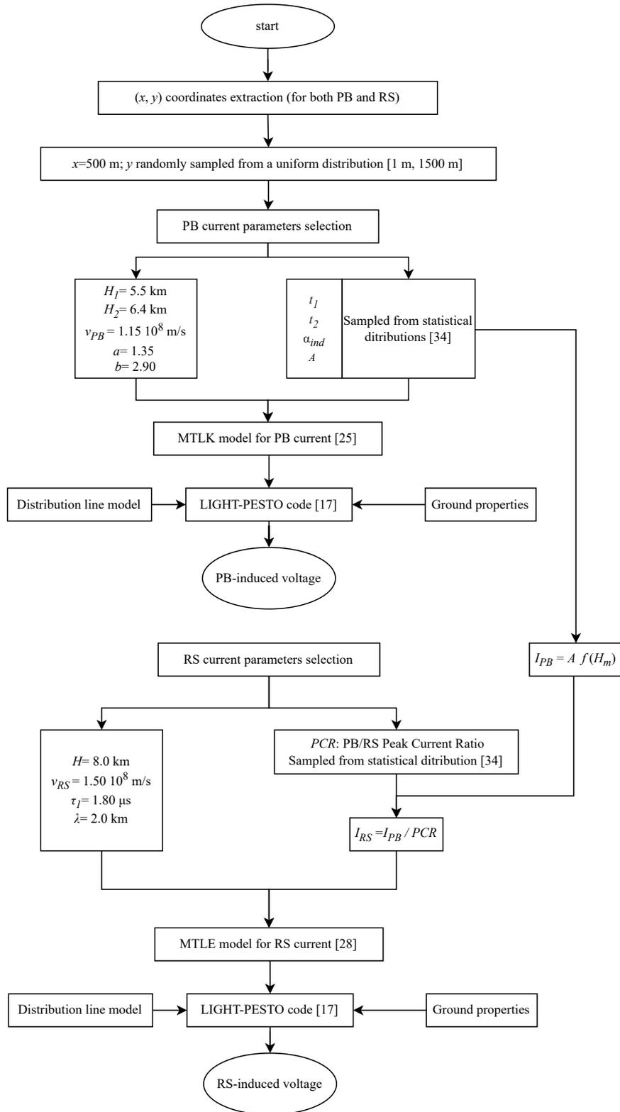
Figure 2: Simulation of voltage waveforms induced by the PB and RS phases of an individual lightning event.
