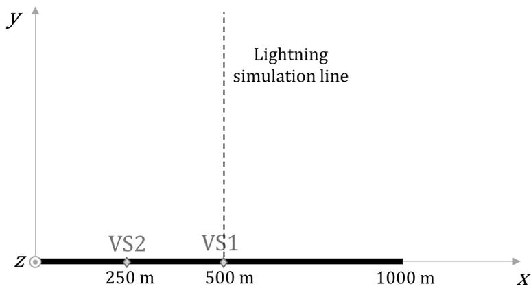
Figure 1: Top view of the modeled network layout. In both scenarios, the phase conductor runs along the plane  $y = 0$  at an height of  $z = 10$  m, with the voltage sensors VS1 and VS2 mounted at positions  $x = 500$  m and  $x = 250$  m. In Scenario B, an additional neutral conductor is present on the same vertical plane, located at  $z = 8$  m.
