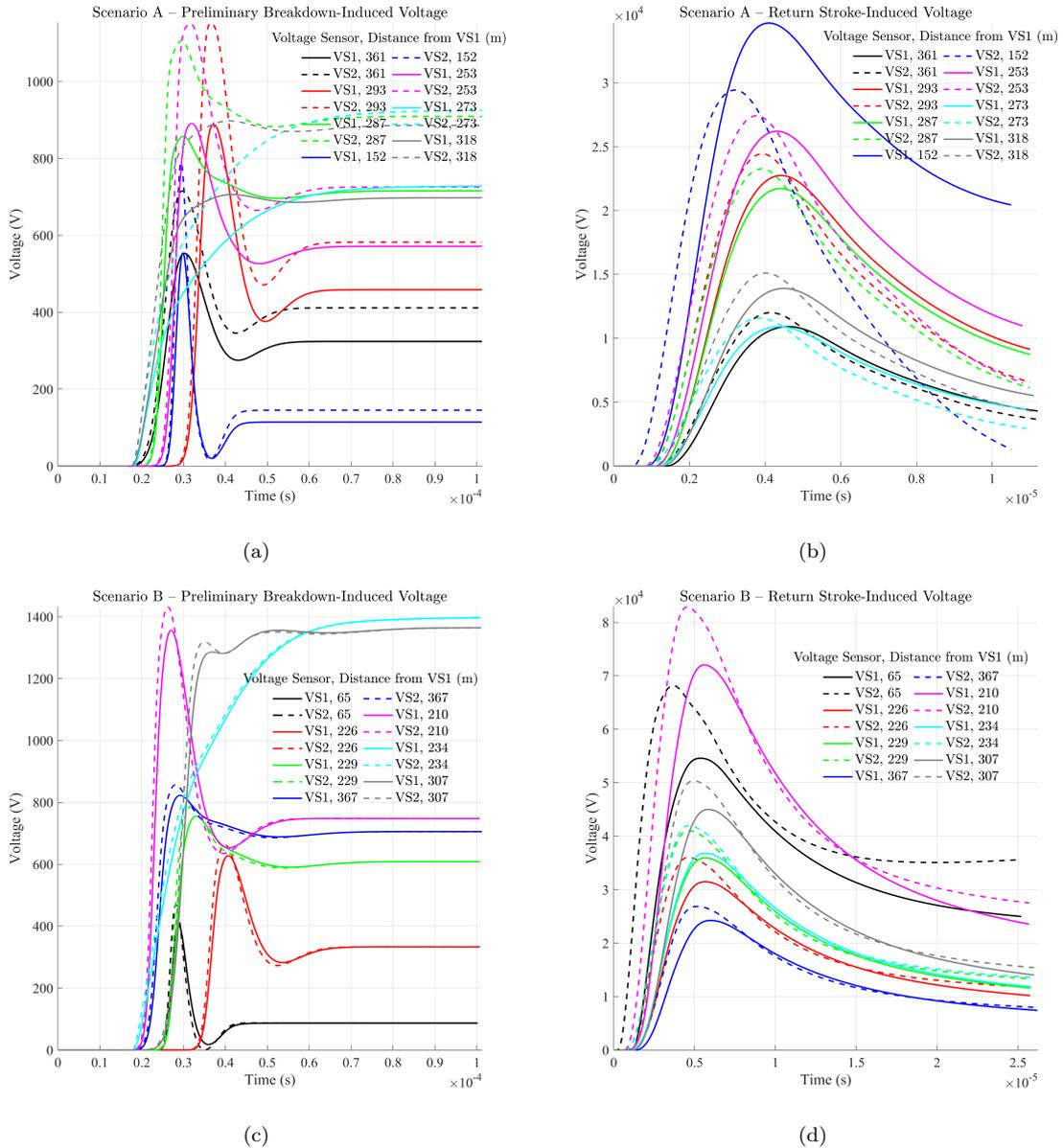
Figure 3: Sample voltage waveforms from the dataset. (a) PB-induced voltages for Scenario A measured at VS1 ( $x = 500$  m) and VS2 ( $x = 250$  m). (b) RS-induced voltages for Scenario A at VS1 and VS2. (c) PB-induced voltages for Scenario B at VS1 and VS2. (d) RS-induced voltages for Scenario B at VS1 and VS2.
